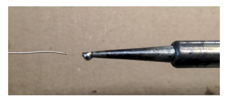
Dip the tip into the dry cleaning sponge once(!!) to remove excess solder, do not thoroughly wipe the tip in the sponge and do not "clean off" the solder too well. The solder is actually good maintenance for the tip, wiping too much off creates microscopic scratches in the tip.
