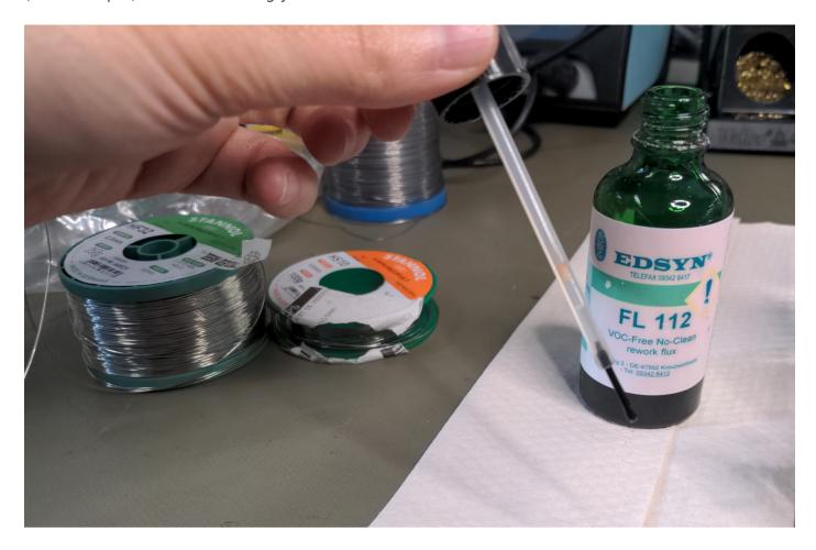
Bigger components like thicker wires or more oxidised surfaces can also require extra flux to be applied. Apply the flux to the component you're struggling with, then hold the iron and solder against to the components or wire. Make sure to shortly remove the iron before applying more flux, you do not want to burn the brush with the iron. Work quickly though, do not let the components cool down too much.
